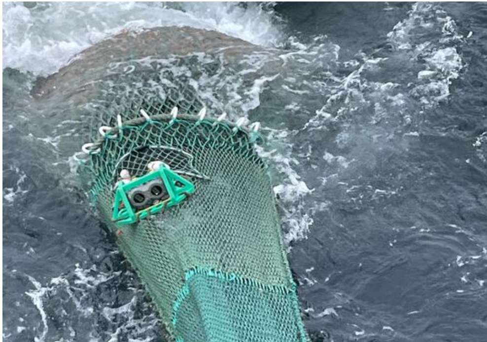
Figure 8. Tunc Grid fitted to a trawl with CatchCam overlooking it.
